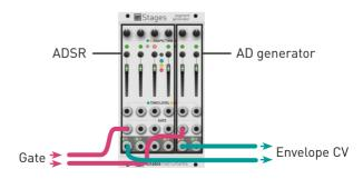
What happens if only **GATE** input 5 is patched? Segments 5 and 6 act as a 2-segment envelope generator; and segments 1, 2, 3 and 4 are four independent free-running generators. Even if these four independent generators do not receive gates or triggers, looping can be enabled for them, turning them, for example, into four LFOs.
