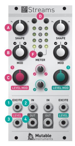
**F. Metering button**. Press to display the bargraph. Press again to select which signal is to be monitored.
